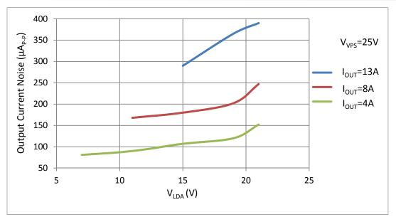
Figure 13. V<sub>LDA</sub> vs. Output Current Noise@0.1Hz~10Hz
