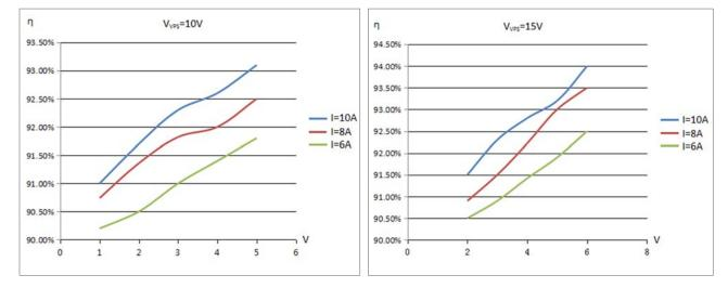
Figure 9. Efficiency of Laser Driver
