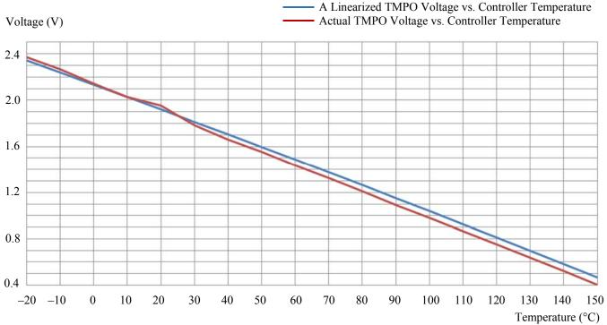
Figure 8. Controller Internal Temperature vs. TMPO Voltage
