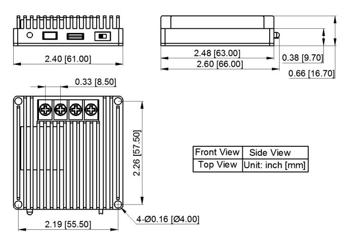
Figure 17. Dimensions of ATLS25A219GUI
