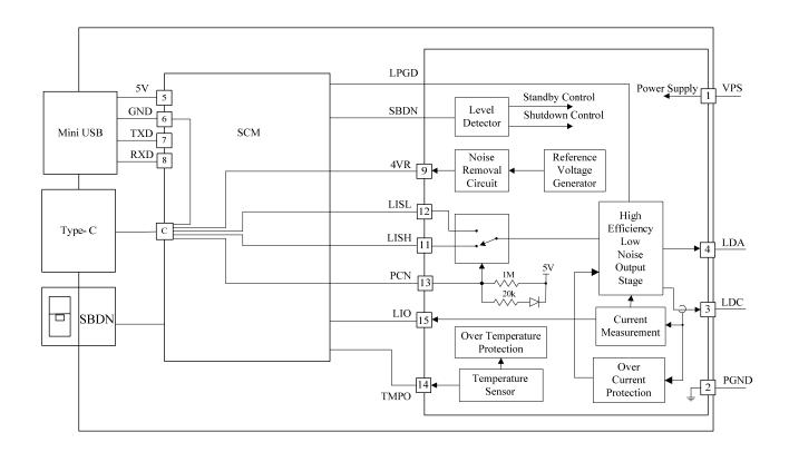
Figure 6. Internal Block Diagram of ATLS25A219GUI
