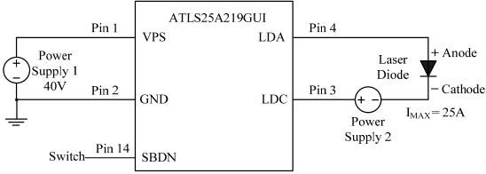
Figure 16. Driving High Voltage Laser Diodes
