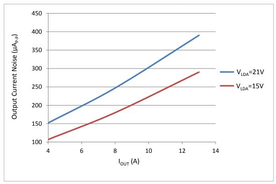
Figure 14. I<sub>OUT</sub> vs. Output Current Noise@0.1Hz~10Hz
