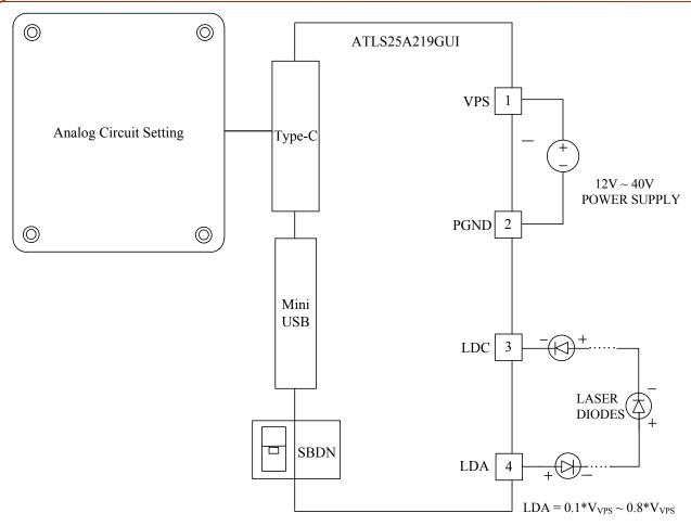
Figure 11. Micro-Controller Based Application Schematic
