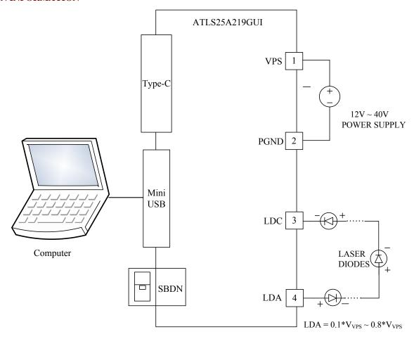
Figure 10. Stand-Alone Application Schematic
