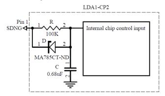
Figure 3. Internal Shut down Circuit
