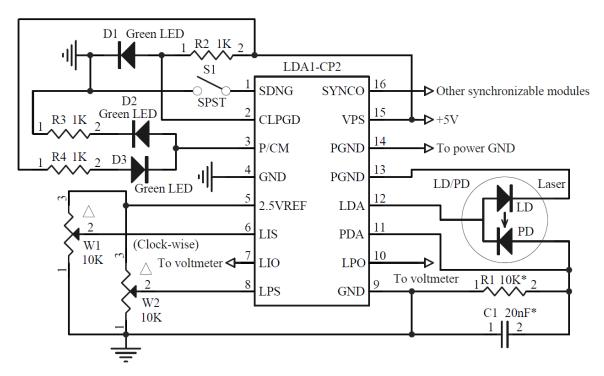
Figure 4. A Typical Self-contained Application Schematic
