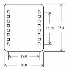
Figure 7. Top View of LDA1-CP2-D
