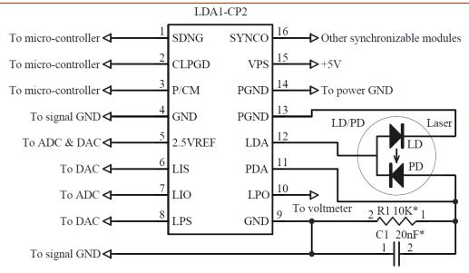
Figure 5. A Typical Micro-processor Based Application
