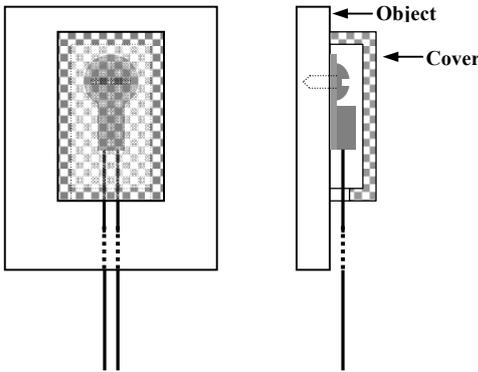
Figure 3. Using an Insulation Cover to Improve Accuracy
