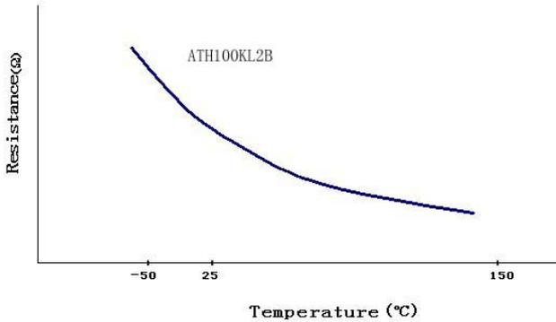
Figure 4. Resistance vs. Temperature for ATH100KL2B
