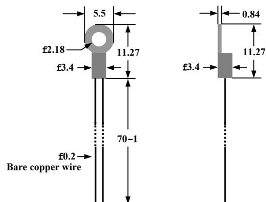
Figure 2. The Front and Side Views of ATH100KL2B
