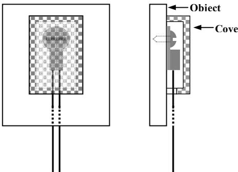
Figure 3. Using an Insulation Cover to Improve Accuracy
