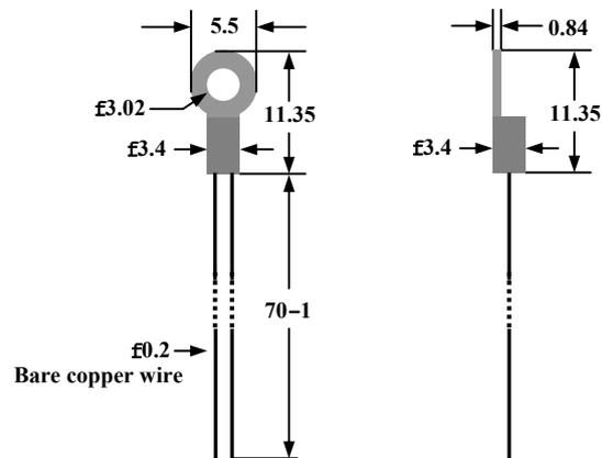
Figure 2. The Front and Side Views of ATH100KL2C
