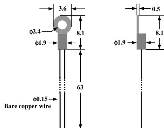
Figure 2. The Front and Side Views of ATH100KL2A
